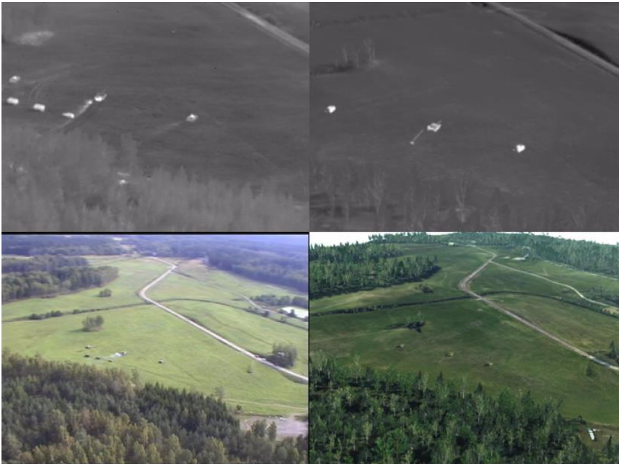
Figure 6: Top: Comparison of an IR-image from a real (left) and simulated (right) QWIP-sensor. Bottom: Same scene but with a visual sensor (left: real, right: simulated).
