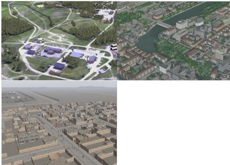
Figure 2: Terrain models in MSSLab: a geospecific Swedish countryside model with forests and open fields, a geospecific Swedish city model with inner city, industrial areas, ports etc., and a geotypical Middle Eastern model with a city and a military camp.
