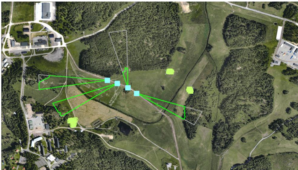
Figure 12: A sensor management example of a reconnaissance group of four vehicles (blue) advances along a road. The current field-of-view of each sensor is illustrated with green lines. Three groups of targets (green), classified as neutral, have been detected.
